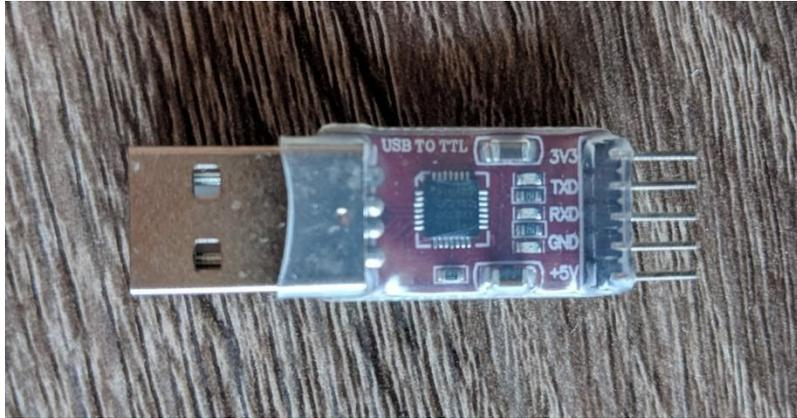
**Figure 3.** USB adapter for serial signals
