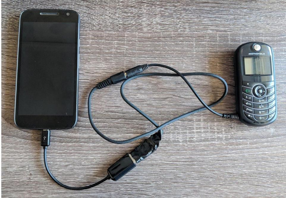
Figure 14. IMSI-Catchers detection sensor.
